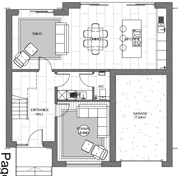
PROPOSED GROUND FLOOR PLAN SCALE 1:50 AREA 70.71m 2
