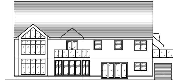
PROPOSED REAR ELEVATION. NORTH FACING.
